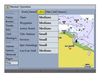
Chart, Waypoints, Active Route, Tide Stations, Services, Spot Soundings, Lat/Lon Grid—controls the screen size of the text for a given map item. Select None, Small, Medium, or Large.
